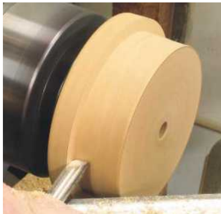
▲ Pic.11 Just like turning a bowl, the majority of the timber is taken away with the 13mm bowl gouge. Here I am just refining a right angle detail with the round parting tool
